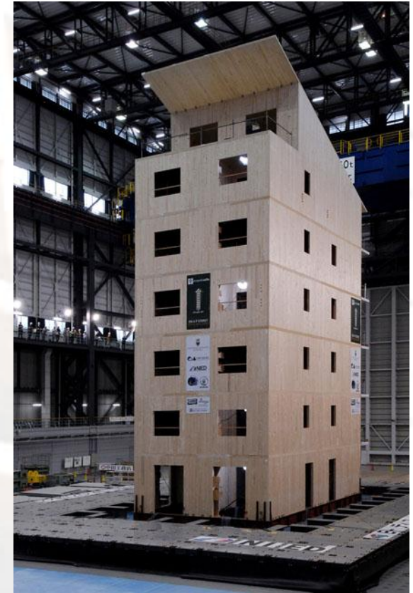
SOFIE 7-storey CLT building test
