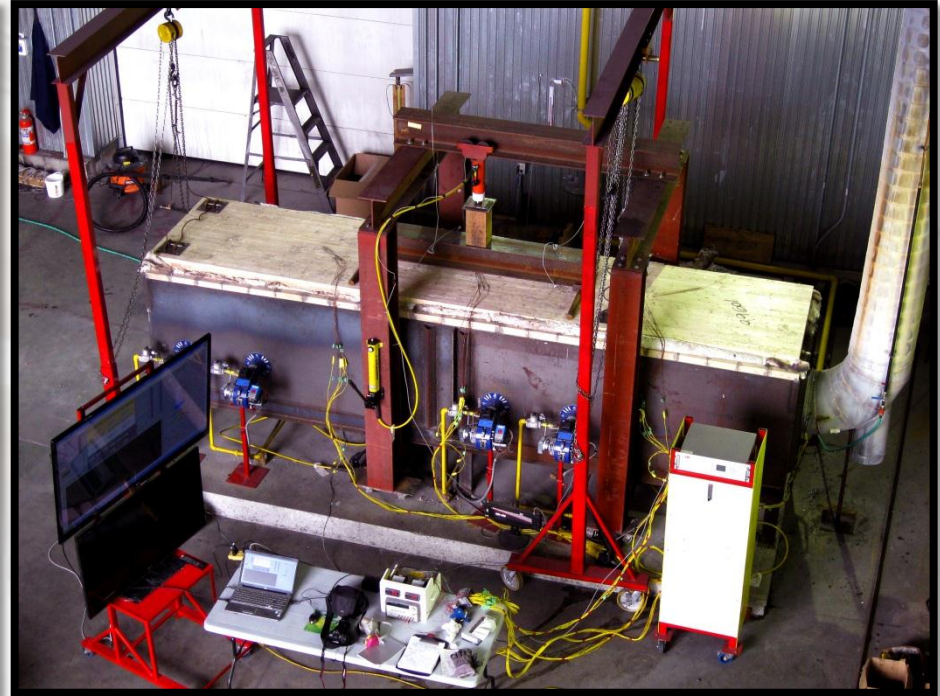
Carleton University Mid-Scale Fire Testing Floor Furnace under 4- point load
