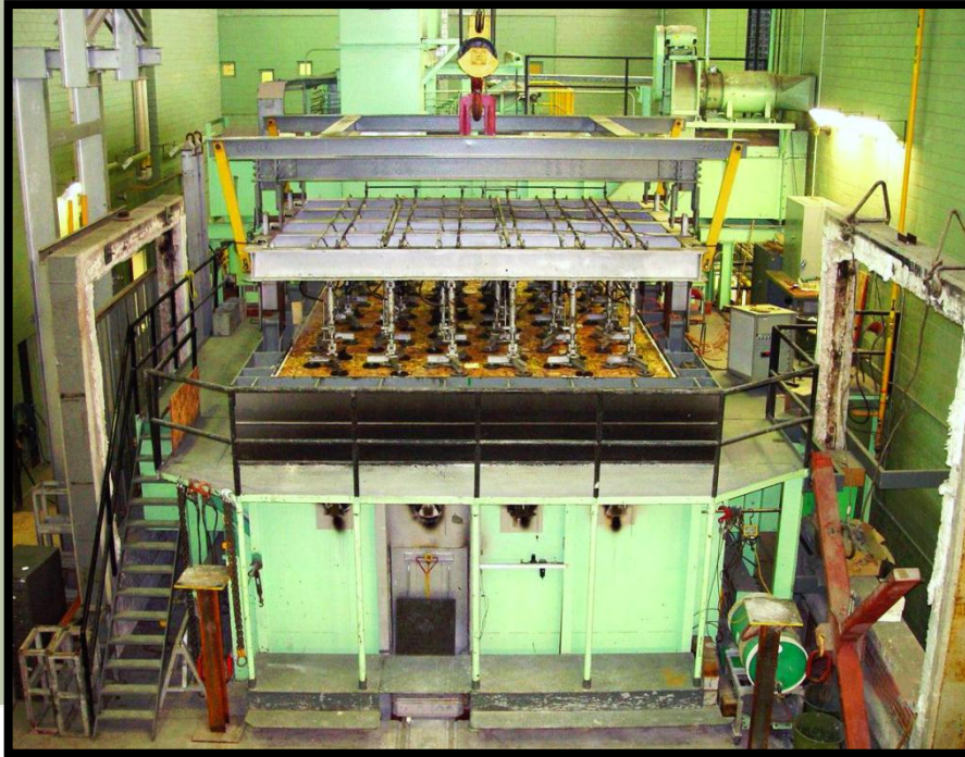
NRC Full-Scale Fire Testing Floor Furnace Under UDL
